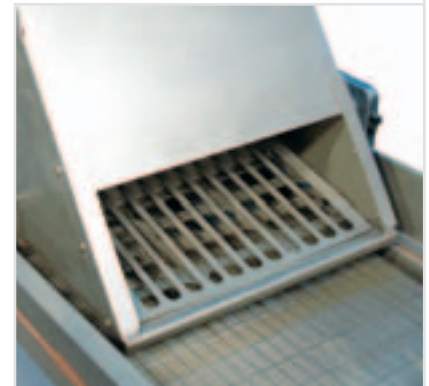
Gumbo slide design minimizes gumbo buildup.
